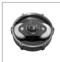
Drive speed reducer and planetary gearbox in oil bath
