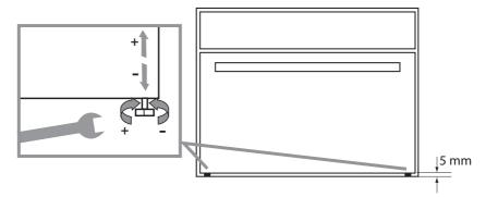
There should be a 5 mm gap between the top of the door glass and the bottom of the control panel. The control panel can be raised or lowered to achieve this gap by first loosening the two screws on either side of the product with a tamper proof torx 20 Screwdriver. Once the control panel is adjusted to suit, ensure the screws are fully tightened again and the panel does not move. This adjustment also allows you to visually align the product incase the cabinetry is not square.
